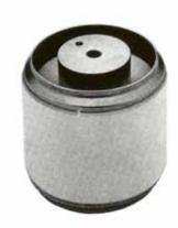
The Y-812 is a planar triode intended for use as a high voltage series regulator or switch tube. The compact, low inductance package allows fast rise and fall times and very short pulse operation. The plate is conduction cooled and rated at 1000 watts when used with the proper heatsink. When immersed in oil the maximum plate voltage rating is 40 kV.
