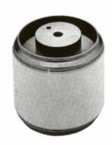
The Y-811 is a planar triode intended for use as a high voltage series regulator or switch tube. The compact, low inductance package allows fast rise and fall times and very short pulse operation. The plate is conduction cooled and rated at 1000 watts when used with the proper heatsink. When immersed in oil the maximum plate voltage rating is 65 kV.
