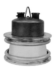
The 8973 is a power tetrode designed for very high powered medium frequency or high frequency broadcast service and a very low frequency communication in the half-megawatt power range. The 8973 has a thoriated tungsten filament mounted on water-cooled supports. Large diameter coaxial terminals are used for the control grid and the RF filament terminals. Filament power and filament support cooling water connections are made through special couplings with threaded clamping rings.
