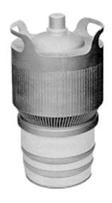
The 4CX5000R/8170W incorporates rugged internal construction features including a sturdy mesh filament which allows it to meet demanding vibration and shock specifications. The 4CX5000R/ 8170W is useful up to 110 MHz and is recommended for use as a radio frequency linear amplifier, a Class AB audio amplifier, or a Class C power amplifier or plate-modulated amplifier.
