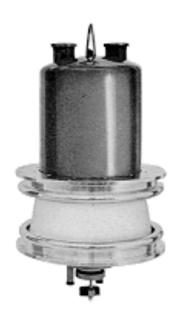
The 4CPW1000KB/X-2062M is a water-cooled power tetrode intended for use as a pulse modulator or pulse regulator. The tube is rated for 175 kVdc holdoff in a protective atmosphere, with a 75 ampere pulse cathode current rating during conduction and a 1000 kilowatt anode dissipation rating (average during the pulse). Peak anode current capability in excess of 100 amperes for short pulse operation is practical.
