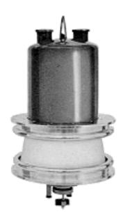
The 4CPW1000KA/9009 is a water-cooled power tetrode intended for use as a pulse modulator or in pulse regulator service. The tube is rated for 150 kVdc holdoff in a protective atmosphere, with a 90 amperes pulse cathode current rating during conduction and a 1000 kilowatt anode dissipation rating (average during pulse). Peak anode current capability in excess of 150 amperes for short pulse operation is practical.
