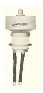
The 3CX5000H3 is a forced air cooled, ceramic/metal, medium-mu triode designed primarily for use in industrial RF heating applications. Input of 23.6 kW is permissible up to 90 MHz. Plentiful reserve emission is available from the 560 watt filament. The grid structure is rated at 150 watts making this tube an excellent choice for industrial service.
