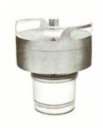
The 3CX5000A7 medium-mu triode is designed primarily for use as a power oscillator in industrial heataing applications. It is also recommended for use as a grounded grid FM amplifier, as a conventional plate modulator or as a linear amplifier. Plentiful reserve emission is available from the 560 watt filament. The grid structure is rated at 100 watts making this tube an excellent choice for severe applications.
