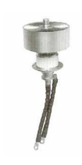
The 3CX4500F3 /YU-108 is a forced air cooled, ceramic/metal, medium-mu power triode designed primarily for use in industrial radio frequency heating services. Input of 24 kW is permissible up to 75 MHz. Plentiful reserve emission is available from it's 546 watt filament. The grid structure is rated at 300 watts making this tube an excellent choice for industrial service.
