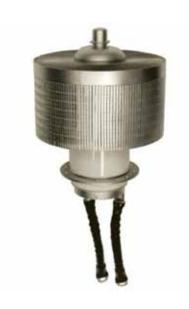
The 3CX20,000H3 is a forced air cooled, ceramic/metal, medium-mu power triode designed primarily for use in industrial radio frequency heating services. Input of 84 kW is permissible up to 90 MHz. Plentiful reserve emission is available from it's 1600 watt filament. The grid structure is rated at 800 watts making this tube an excellent choice for industrial service.
