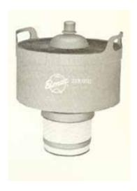
The 3CX20,000A3 is a forced-air cooled, ceramic/metal, medium-mu power triode designed primarily for use in industrial radio frequency heating services. Input of 84 kW is permissible up to 90 MHz. Plentiful reserve emission is available from its 1600 watt filament. The grid structure is rated at 800 watts making this tube an excellent choice for industrial service.
