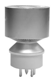
The 3CX1500D3 is a forced-air cooled, ceramic/metal medium-mu triode designed primarily for use in industrial RF heating services. Input of 4.3 kW is permissible up to 110 MHz. Plentiful reserve emission is available from its 158 watt filament. The grid structure is rated at 75 watts making this tube an excellent choice for industrial service.
