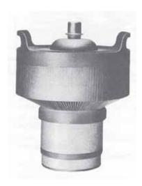
The 3CX15,000A3 is a medium-mu power triode designed for use as a power oscillator in industrial radio frequency heading applications. It is also recommended for use as a conventional plate modulated amplifier or as a linear amplifier. The one kilowatt filament and rugged 500 watt grid structure make this tube especially suited for heavy duty service.
