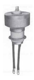
The 3CX10,000H3 is a forced-air cooled, ceramic/metal medium-mu power triode designed primarily for use in industrial RF heating services. Input of 32 kW is permissible up to 90 MHz. Plentiful reserve emission is available from its 743 watt filament. The grid structure is rated at 250 watts making this tube an excellent choice for industrial service.
