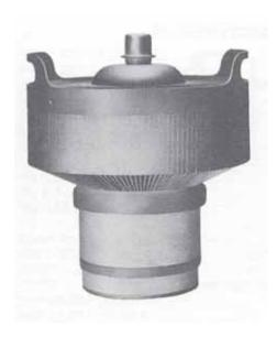
The 3CX10,000A3/8159 is a forced-air cooled, ceramic/metal, medium mu power triode designed primarily for use in industrial radio frequency heating services. Input of 32 kW is permissible up to 140 MHz. Plentiful reserve emission is available from it's 743 watt filament. The grid structure is rated at 250 watts, making this tube an excellent choice for industrial service.
