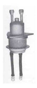
The 3CW10,000H3 is a water-cooled, ceramic/metal, medium-mu power triode designed primarily for use in industrial RF heating services. Its water-cooled anode is conservatively rated at 10 kW of plate dissipation with low water flow and pressure drop. Input of 30 kW is permissible up to 90 MHz. Plentiful reserve emission is available from its 560 watt filament. The grid structure is rated at 150 watts making this tube an excellent choice for industrial service.
