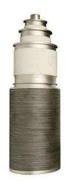
The ML-6697A is a forced-air cooled ceramic/metal triode designed for AM broadcast and communications amplifiers and for industrial heating service. The heavy wall anode with high efficiency disc fins is capable of dissipating 35 kW. The ML-6697A will operate with plate voltages up to 16 kV in CW operation. Maximum ratings apply at frequencies up to 40 MHz. Useful power output can be obtained at frequencies up to 80 MHz with reduced ratings.
