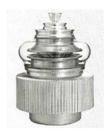
The LPT-62 is a ruggedized version of the ML-7715. It is a shielded-grid triode designed primarily for use as a switch tube in hard-tube pulse modulators for radar applications. It can deliver a peak pulse power output of 3.5 MW with less than 7 kW driving power. The maximum ratings of 65 kVdc and 70 kW peak apply when the tube is completely immersed in a suitable dielectric fluid such as sulfur hexafluoride or a mineral oil.
