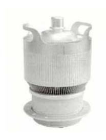
The Eimac YC-156A is a rugged ceramic/ metal high-mu power triode designed for pulsed rf applications. Utilizing beamforming cathode and control grid geometry, this tube provides the gain of a tetrode with circuit advantages and simplified design of a triode. The attributes of high gain, low grid interception and outstanding intermodulation performance make this tube well suited for application such as MRI and pulsed linear amplifier service.
