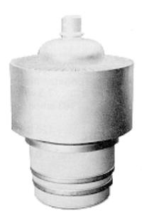
The 4CX7500A is a compact tetrode designed to be used in VHF power amplifer service. It features a type of internal structure which results in high RF operating efficiency up to 220 MHz. A dense mesh filament is used which contributes to the high performance capability of the tube. This tube is also recommended for use as a VHF TV linear amplifier.
