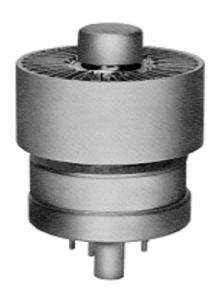
The 4CX350AC/8321A is a compact air cooled tetrode. This tube is intended for use in equipment which normally uses the 4CX350 and where extended tube life is a concern. Externally the 4CX350AC/8321A is identical to the 4CX350A. Electrical characteristics are the same in both tube types with the exception that the heater warm-up time is increased to 40 seconds in the 4CX350AC/8321A.
