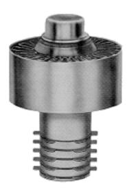
The 4CX300A/8167 is a compact power tetrode having a maximum plate dissipation rating of 300 watts. The ceramic/metal construction and the internally utilized electrode structure combine to make the 4CX300A/8167 especially durable and free from mechanically induced noise under conditions of severe acceleration caused by shock and vibration.
