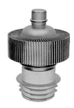
The 4CX1500A is a general purpose tetrode for use up to and through VHF. Insulation is ceramic and the thoriated tungsten filament is a rugged mesh design. The screen terminal is a continuous ring which allows good isolation between the plate and the control grid circuit. The 4CX1500A is recommended for use as a Class C power amplifier, Class B or Class AB1 linear amplifier, and as a regulator and in pulse modulator service.
