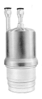
The 4CW10,000A/8661 is electrically identical to the 4CX10,000D/8171 and 4CX5000A/8170 except for its plate dissipation, which is rated at 12 kW. The tube is useful up 10 110 MHz and is suggested for general use as an oscillator, amplifier or modulator. A pair of these tubes will deliver more than 30 kW of audio output.
