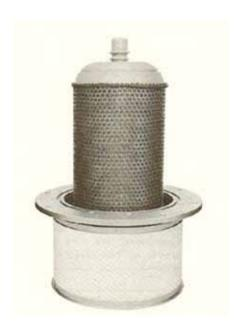
The 4CV100,000E is recommended for use as a Class C RF amplifier, a Class AB RF amplifier, a Class AB push-pull AF amplifier or modulator, as well as a high level modulated or pulse duration modulated amplifier. The tube is characterized by low input and feedback capacitances and low internal lead inductance. A rugged thoriated tungsten mesh filament provides ample emission over long operating life.
