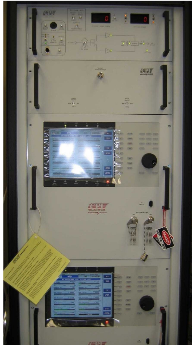
CPI 900 W S/C-band TWTA System, Model VZSC2780P2
