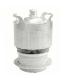
The 3CPX5000A7 high-mu triode is designed for use as a cathode driven Class AB pulsed power amplifier and as a switch tube in cathode or grid drive service. The tube does not require a socket as it is designed to bolt directly to the chassis by means of the grid flange. Cathode and heater connections are made by bolting directly to the amplifier circuitry. These features reduce equipment cost and complexity.
